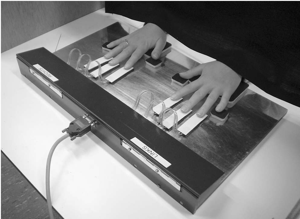
Figure 3. The experimental setup. The positions of the stimulus elements could be adjusted to the positions of the fingers of the participant. Under each element was a sensor that measured whether a finger was on top of it.
